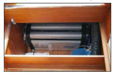
This photo shows the main part of the water maker, installed in the locker space revealed by sliding the portside step inwards. Running it consists of turning on the power, flushing it for 3-4 mins to avoid the saltiness that comes through as it first pressurises. Then, turning the three way
